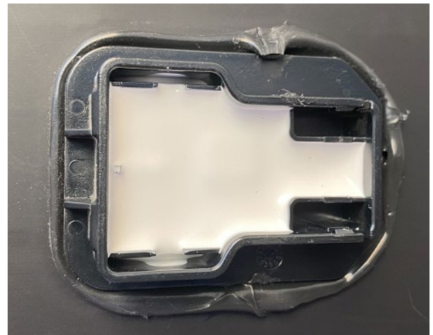
Junction box (opened)
