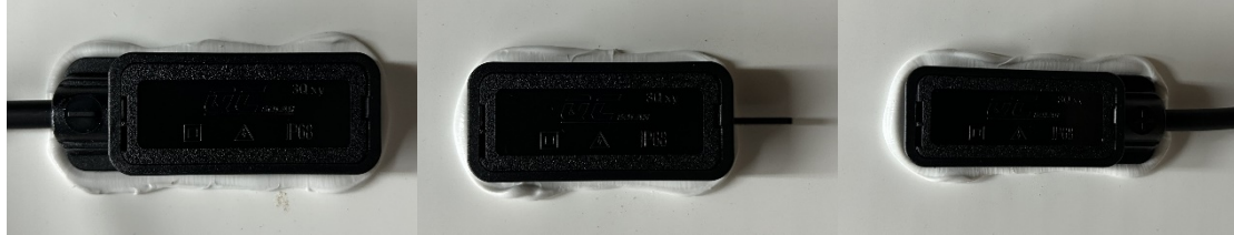
Fig. 3: View of junction box of module type SR-72M600NHLPro
